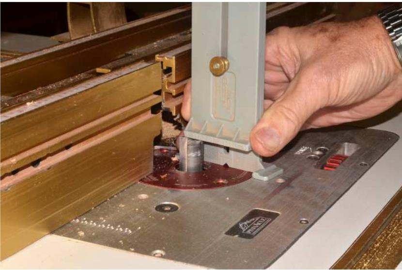
Of course, just like setting the table saw blade height, I use the Incra Gauge to set the bit height at the router table as well. (And no, I am not planning on making that deep a cut in a single pass. It was just easier to photograph the gauge in use by raising the bit that high).
