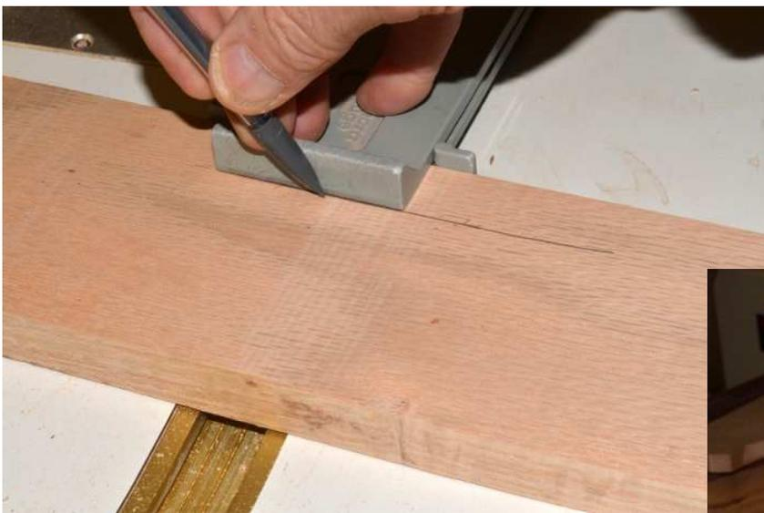
The Incra Gauge is also a useful tool for locating from the edge of a work piece. It slides easily so one can mark along an edge, or, use it to position another piece, (such as the drawer pull shown in the photo below).
