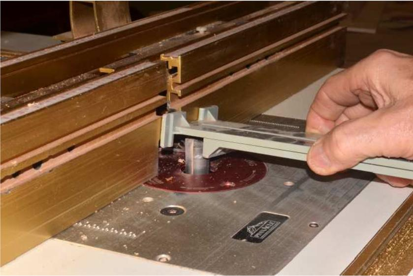
Accurately locating the router table fence for a dado or other cut is also easy. In this photo I want a 3/4" dado 1/2" from the edge of the workpiece. I set the Incra Gauge to 1 1/4", move the fence in place and lock it there. The cut is right where I need it.
