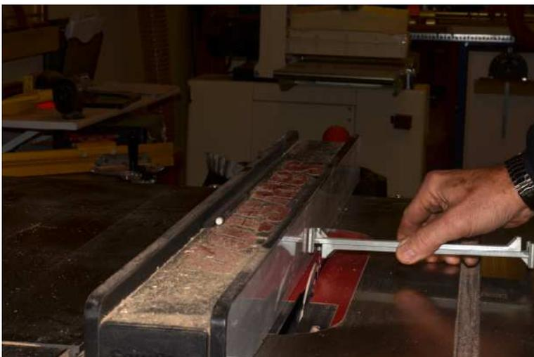
Use it also to set the distance from the fence. I use the combination of this measurement along with setting the height as shown above, to cut a clean, accurate rabbet in two passes. I especially like that approach over using the router table with woods that like to chip and splinter when using a rabbeting cutting on the router.
