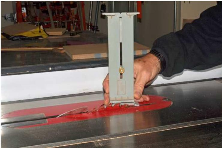
Use it to set the height of the table saw blade. This is particularly useful when I am sawing off the lid of a box I am making. I want to saw all the way through the two long size, and then leave no more than a  $1/32$ ” web on the two short sides, that I cut through at the bench. The Incra gauge with its milled accuracy to  $1/32$ ” lets me get that level of precision.
