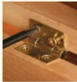
**Square the corners and install the hinges.** The router bit leaves rounded corners, so you'll need to square them with a chisel. The fit will be perfect.
