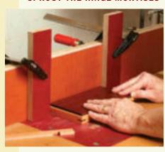
Mortise in two steps. With the stop blocks in place, cut one mortise in the lid and a second on the box. Flip the stick and reposition the stop blocks; then cut the remaining mortises on the lid and box.
