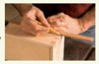
Notch the stick. Stowe uses his tablesaw to cut a precise notch to accept the leaves of the hinge.
